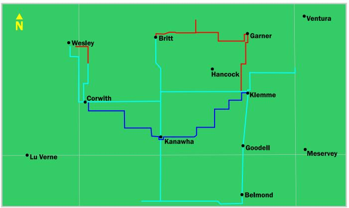
Comm1 has installed a state-of-the-art fiber ring between the communities we serve. This ring is connected to the statewide fiber network managed by Iowa Network Services. It gives us the ability to offer a redundant fiber connection between the communities we serve and major cities in our region.
